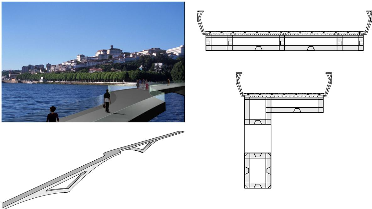
Fig. 2 - Perspectives of the footbridge. Cross-sections at mid-span and at in the proximity of the arch springs
