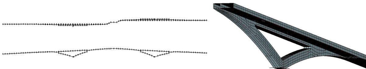
Fig. 3 - Plan and side view of the beam finite element mesh. Detail of shell finite element model
