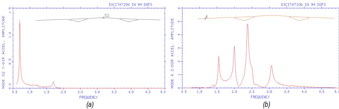
Fig. 6 - Spectral acceleration associated uniformly distributed pedestrian load (1person/m<sup>2</sup>): (a) lateral acceleration at mid-span; (b) vertical acceleration at mid-point of transition span (m/s<sup>2</sup>)
