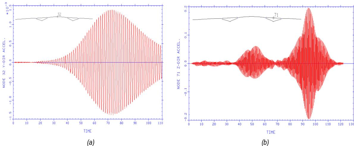
Fig. 5 - Response history associated with single pedestrian propagation: (a) lateral acceleration at mid-span for  $f_p=0.704\text{Hz}$ ; (b) vertical acceleration at mid-point of tie for  $f_p=2.522\text{Hz}$  (m/s<sup>2</sup>)
