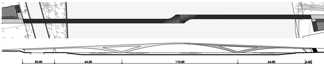
Fig. 1 - Plan view and elevation of the footbridge
